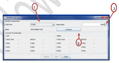
Press **Connect.** Wait to be sure the instrument is connected.
